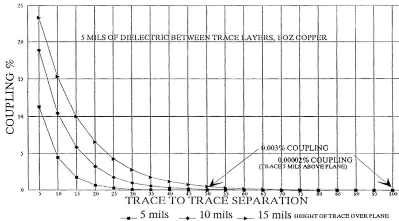
FIGURE 13.7 Trace-to-trace coupling. (Prepared by Shared Resources, Inc.)
