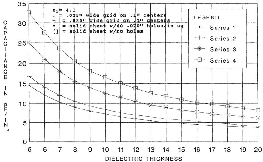
FIGURE 13.14 Capacitance per unit area vs. dielectric thickness.
