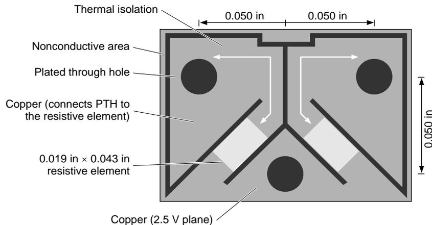
**FIGURE 13.13** The two light diagonal shapes in the figure above are terminating resistors for ECL transmission lines. They are formed directly in the VTT powerplane by etching the copper away from the underlying nickel resistive layer. One end of each resistor is connected to the device terminal using a via and the other end is connected directly to the -2.5V plane. (Courtesy of Ohmega Industries.)
