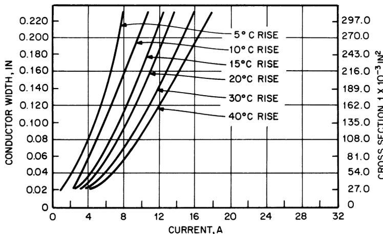
FIGURE 13.5 Temperature rise vs. current for 1-oz copper.
