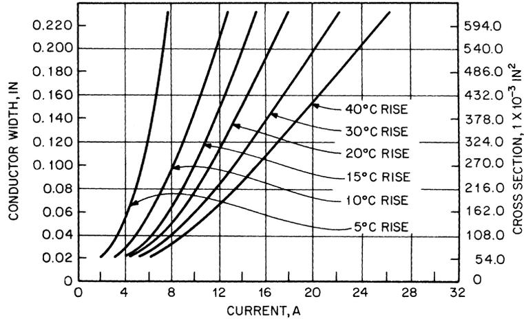
FIGURE 13.6 Temperature rise vs. current for 2-oz copper.
