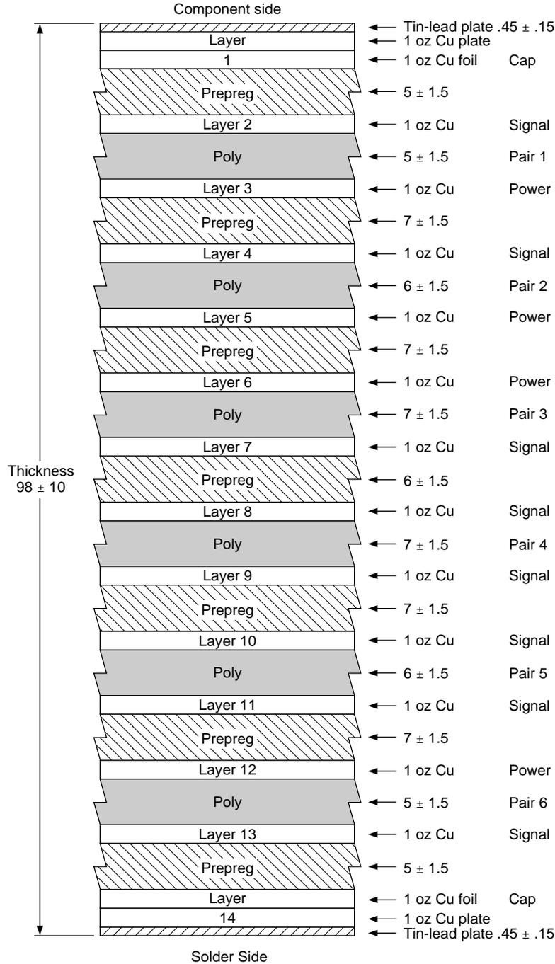
**FIGURE 13.9** Cross section of 14-layer multilayer printed wiring board, showing a typical inner layer and prepreg material relationship. In this case, to reduce z-axis expansion, the innerlayers are polyimide, while the prepreg material is semicured polyimide. Typical signal, power, and ground layers are also indicated, as well as the thickness of the copper foil for each layer.
